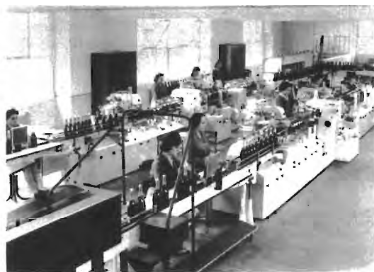
Modern equipment for labelling bottles (Delavaud)
