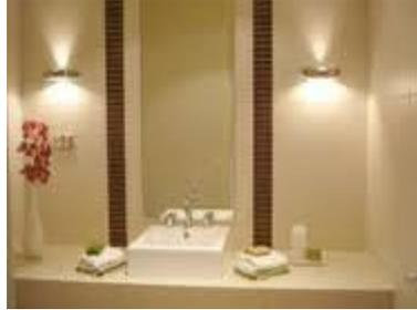
**Diffused lighting-** it is where the bulb or the light source is completely enclosed & lights are diffused through a translucent shade or material.
